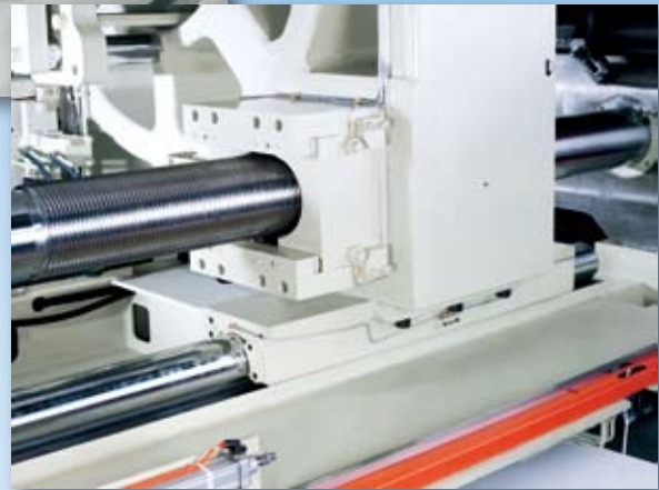
Guide column support mechanism for the Moving Platen, Suitable for SM1200-SM3200
